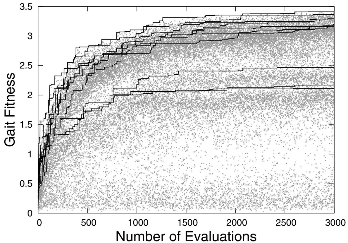
Fig. 6. Ten gait optimization runs. Grey crosses represent evaluated gaits, and black lines indicate the best found so far in each run.
